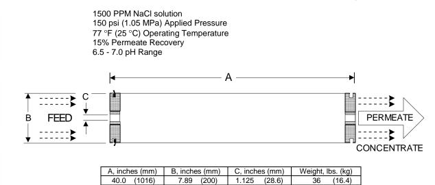
Notice: Permeate flow for individual elements may vary + or - 15 percent. Membrane active area may vary +/-4%. All membrane elements are supplied with a brine seal, interconnector, and o-rings. Elements are enclosed in a sealed polyethylene bag containing less than 1.0% sodium meta-bisulfite solution, and then packaged in a cardboard box. All elements are guaranteed 99.5% minimum rejection.
